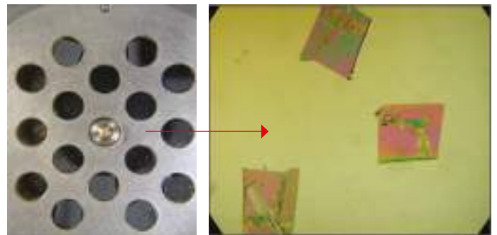
«Harvard» holder with 16 holes and image of microtomed sections of resin-embedded tissues deposited on a 5x5mm silicon square.
